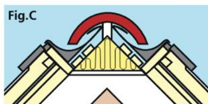
Keylite ridge flashing required
