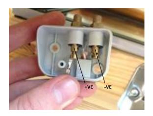
15. Feed the blind wires through the hole in the underside of the Blind Contact. Feed the exposed wire ends through the holes in the contact points and tighten the screws to hold the wires in place.
