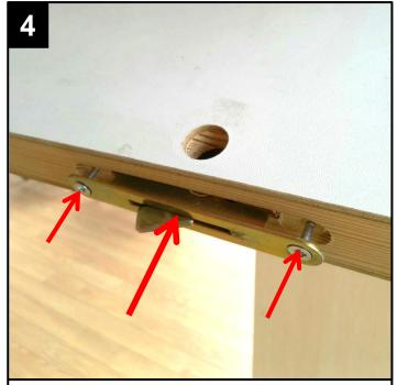
Place the new lock into position and secure in place with the two screws.
