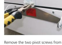
Remove the two pivot screws from the lower part of the transit plate and retain for future use.
